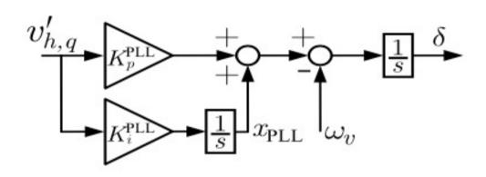
$$\overline{v}_h = \exp(\jmath \, \delta) \, \overline{v}_h' \,, \qquad \overline{\imath}_h = \exp(\jmath \, \delta) \, \overline{\imath}_h'$$
