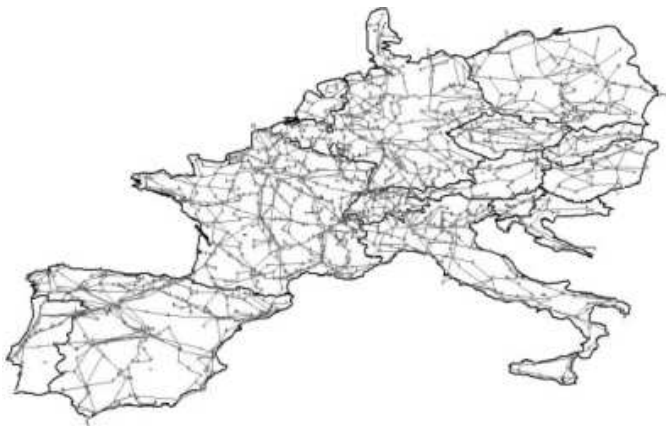
Fig. 1. One-line diagram of the 1254-bus 1942-line model of the UCTE system.
