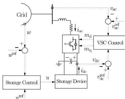
Fig. 1: VSC-based ESS coupled to the grid.
