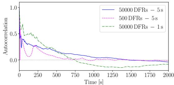
Fig. 9: Effect of clustering on the autocorrelation of a single DFR.
