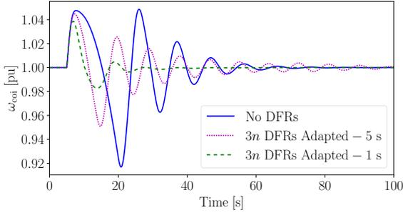
Fig. 4: WSCC 9-bus system – Sensitivity of the stochastic control of DFRs to the operation time interval.
