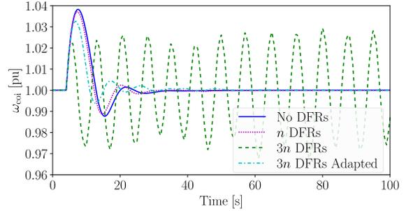
Fig. 7: Frequency response of the all-island Irish system for an operating condition with 30% less inertia than in the base case scenario.
