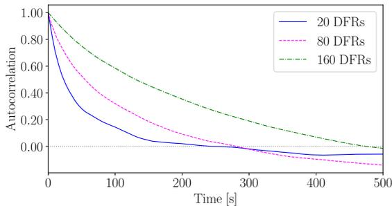
Fig. 5: WSCC 9-bus system – Sensitivity of the autocorrelation of the stochastic behaviour of a DFR to the number of DFRs present in the system.
