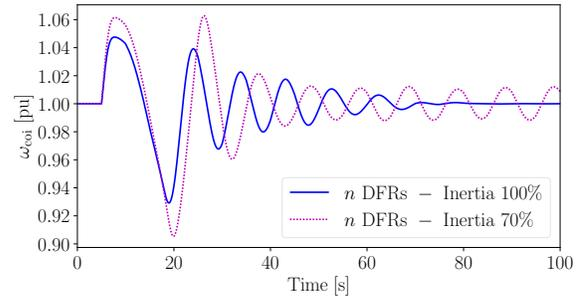
Fig. 2: WSCC 9-bus system – Sensitivity of the stochastic control to the inertia of the system.
