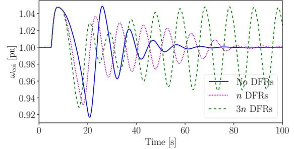
Fig. 1: WSCC 9-bus system – Sensitivity of the stochastic control to the number of DFRs.
