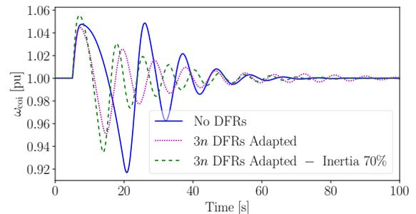
Fig. 3: WSCC 9-bus system – Adaptive stochastic control responding to the change of the number of DFRs and inertia of the system.
