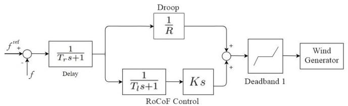
Fig. 1. Block scheme for droop and RoCoF control.
