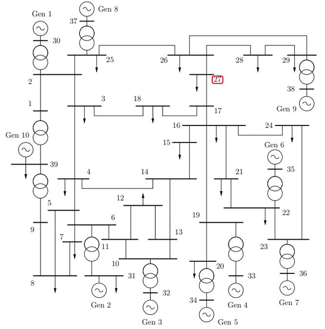
Fig. 4. Scheme of the New England 39-bus 10-machine system [18].
