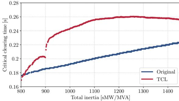
Fig. 8. The CCT values when varying the equivalent inertia of the New-England test system with wind turbines without frequency control and TCLs.
