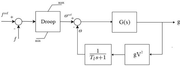
Fig. 3. Block diagram of thermostatically controlled loads used in the case studies.
