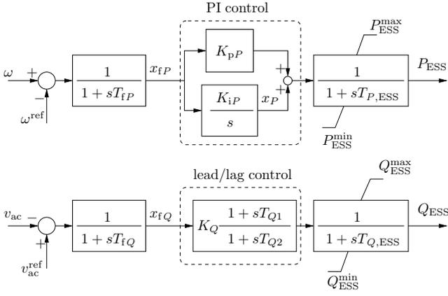
Fig. 2. Block diagram of the simplified ESS model used in the case studies.
