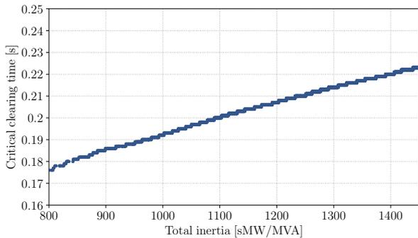
Fig. 5. The CCT values when varying the total equivalent inertia of the original New-England system.
