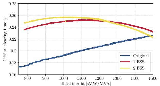
Fig. 7. The CCT values when varying the equivalent inertia of the New-England system including ESSs.
