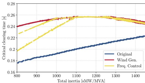
Fig. 6. The CCT values when varying the equivalent inertia of the New-England system including wind turbines with and without frequency control.
