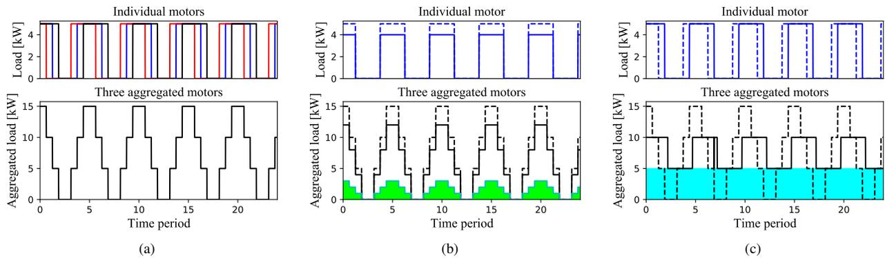
Fig. 14. Three applications with 5kW aggregated in (a) a basic operation, (b) a power shift of 20% enabling a varying flexibility reserve across selected intervals, and (c) a time shift across all applications enabling a continuous flexibility reserve of 5kW.
