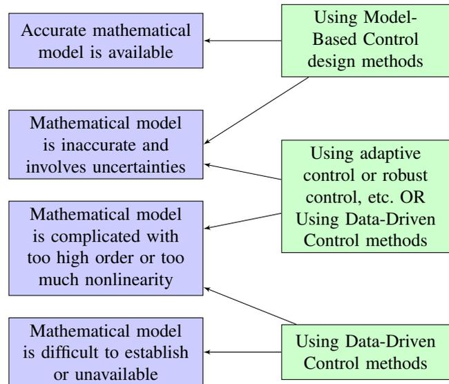
Fig. 12. Choice between Model-Based Control and Data-Driven Control [126].
