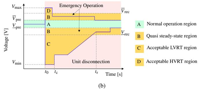
Fig. 6. Example of DER support regions with grid fault occurring at  $t_0$ : (a) Frequency Ride Through (FRT) and (b) Voltage Ride Through (VRT).
