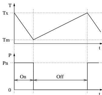
Fig. 20. Temperature and power cycles of a typical refrigerator.
