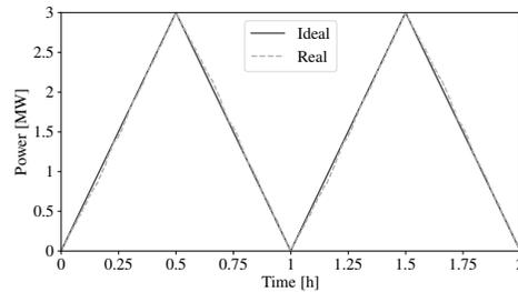
Fig. 22. Total active power consumption of 1000 heat pumps with  $d = 50\%$ .
