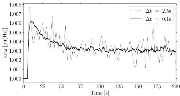
Fig. 23. Effect of the time periods between loads switches on the dynamic performance of the system [148].
