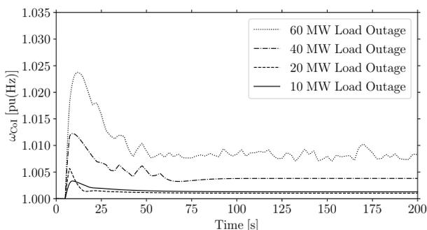
Fig. 24. Clusterized frequency load control combined with ESSs [148].
