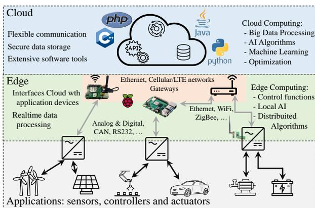
Fig. 13. A diagram depicting a generic arrangement with edge devices and different applications, interfacing with a cloud platform.
