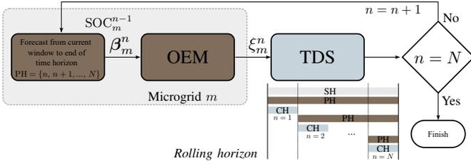
Fig. 2. Flowchart of the testing methodology considering a rolling horizon framework.
