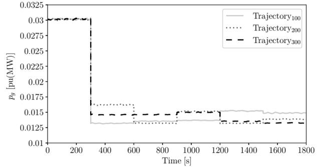
Fig. 10. Active power of MG connected at bus 4 for greedy approach.
