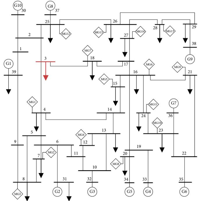
Fig. 3. IEEE 39-bus system with 15 microgrids.
