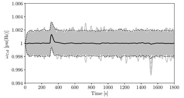
Fig. 9. Frequency of the CoI for the greedy approach. The grey lines represent each realization, the black thick line represents the average of the process, while the dotted line represents the average  $\pm 3$  times the standard deviation.
