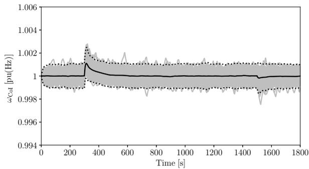
Fig. 11. Frequency of the CoI for the cooperative approach. The grey lines represent each realization, the black thick line represents the average of the process, while the dotted line represents the average  $\pm 3$  times the standard deviation.
