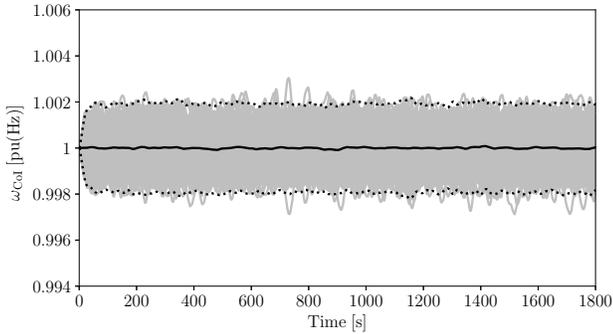
Fig. 8. Frequency of the CoI for the case without MGs. The grey lines represent each realization, the black thick line represents the average of the process, while the dotted line represents the average  $\pm 3$  times the standard deviation.
