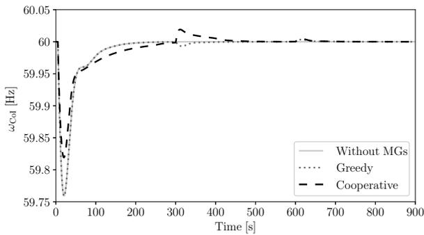
Fig. 4. Frequency response of the conventional scenario.
