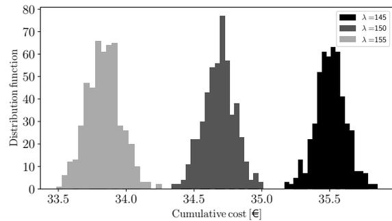
Fig. 13. Histogram of operation cost for different imbalance prices – MG8.
