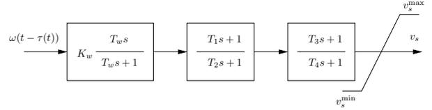
Figure 3: Power system stabilizer control diagram [17].
