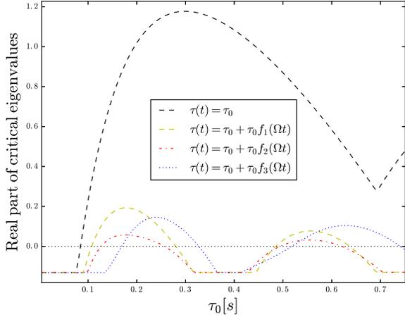
Figure 4: Real-part of the rightmost eigenvalues of the IEEE 14-bus system with 20% load increase as a function of  $\tau_0$ .
