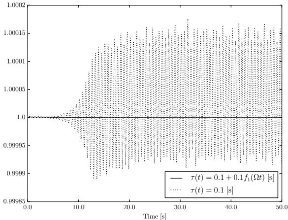
Figure 5: The transient behaviour of bus-1 generator rotor speed of the IEEE 14-bus system with 20% load increase after a small disturbance.
