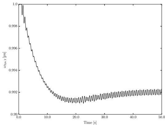
a) Rotor speed of bus-2 generator
