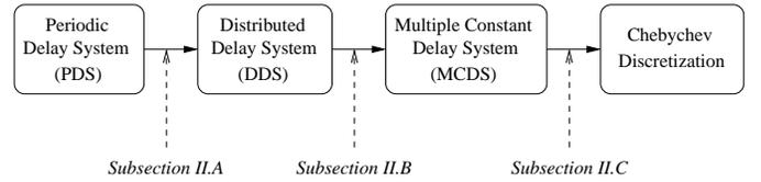
Figure 1: Proposed approach to transform a set of equations with time-varying delays into an equivalent set of equations with multiple constant delays, which is finally linearized and discretized to allow solving the small-signal stability analysis.
