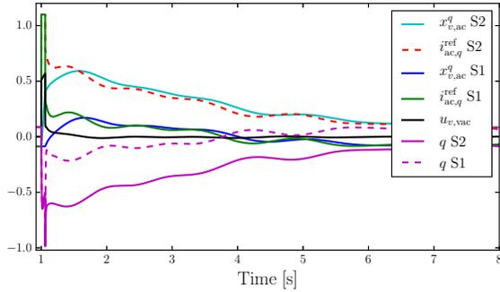
Fig. 11: Scenario (b): Response of the AC voltage controller of the outer level and reactive power support provided by the STATCOM, using models PI2-S1 and PI2-S2.
