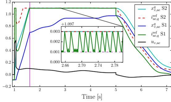
Fig. 10: Scenario (a): Response of the AC voltage controller of the outer level of the STATCOM, using models PI2-S1 and PI2-S2.
