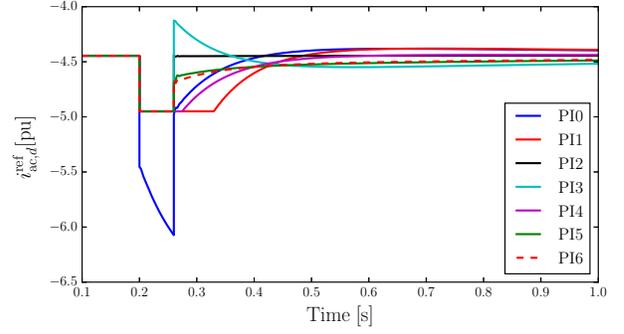
Fig. 7: Response of the output of the active power controller of the Irish-side VSC.
