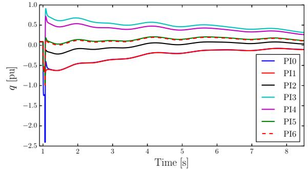
Fig. 13: Scenario (b): reactive power support from STATCOM, using models PI0 to PI6.
