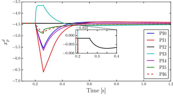
Fig. 5: Response of the integrator state ( $x_p^d$ ) of the active power controller of the Irish-side VSC.
