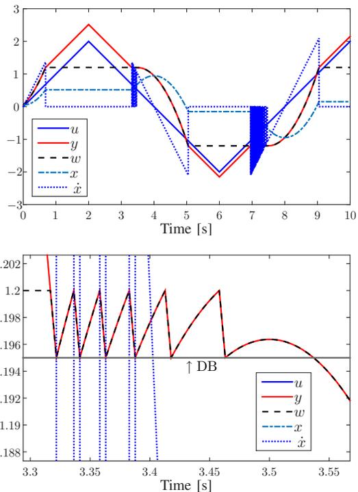
Fig. 2: Simple example to explain the deadlock phenomenon that occurs with the PI2 model.
