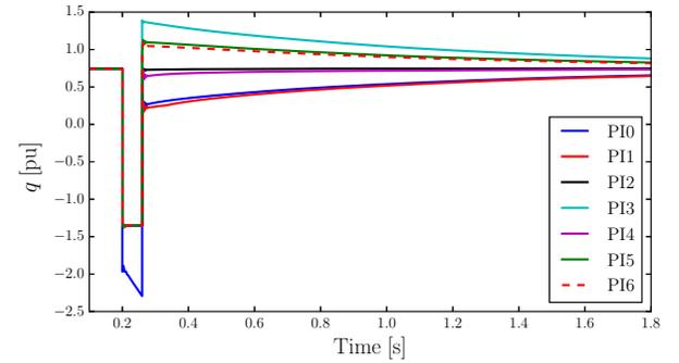
Fig. 9: Response of the reactive power support of the Irish-side VSC.
