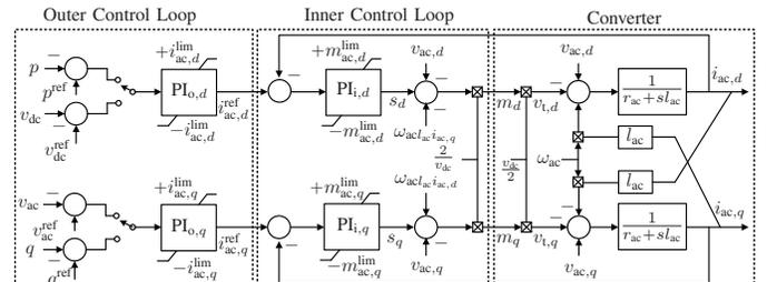
Fig. 4: VSC converter, outer control and inner current control in  $dq$ -frame.
