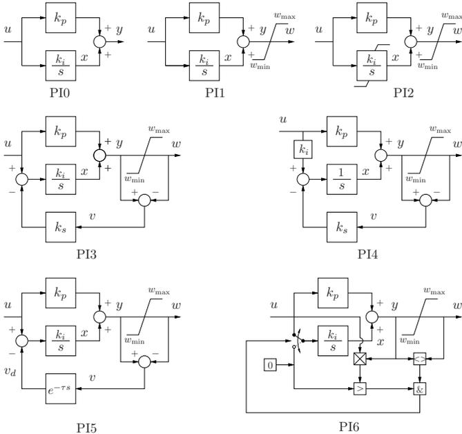
Fig. 1: PI models: (PI0) no limits; (PI1) windup limiter; (PI2) IEEE Standard 421.5-2016 with conditional integrator; (PI3) back calculation type I, (PI4) back calculation type II; (PI5) back calculation with delay; and (PI6) combined conditional and back calculation.
