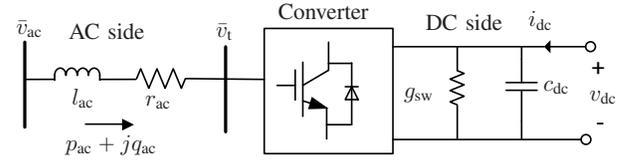
Fig. 3: VSC scheme interfacing a DC grid with an AC grid.
