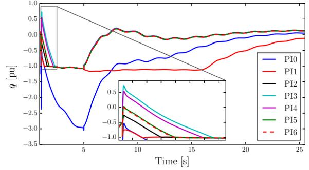
Fig. 12: Scenario (a): reactive power support from STATCOM, using models PI0 to PI6.
