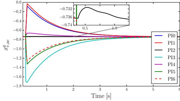
Fig. 6: Response of the integrator state ( $x_{v,ac}^q$ ) of the AC voltage controller of the Irish-side VSC.
