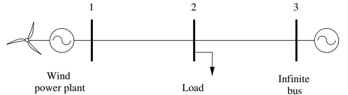
Fig. 1: The OMIB test system.
