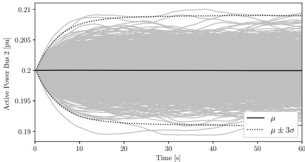
Fig. 3: Illustration of Method II. In this case the processes reach stationarity at time 20 s. From there on, the standard deviation is not continuously growing.
