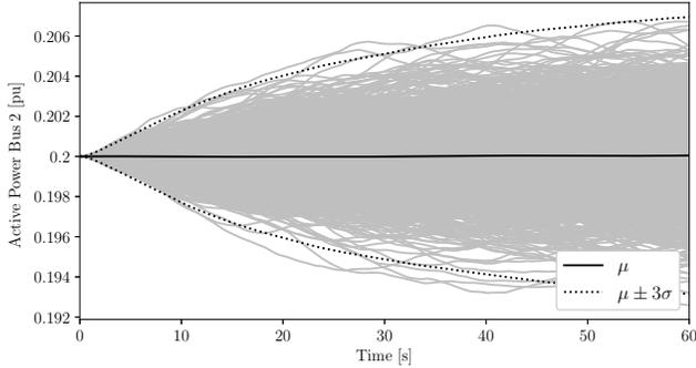
Fig. 2: Illustration of Method I. In this case the stochastic processes have not reached stationarity as the standard deviation is still continuously growing at time 60 s.
