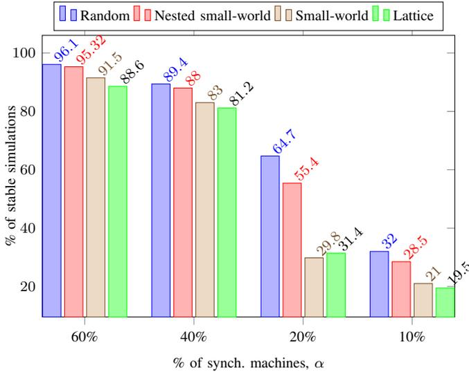
Fig. 2: Transient stability analysis: percentages of stable simulations following a three-phase short-circuit.
