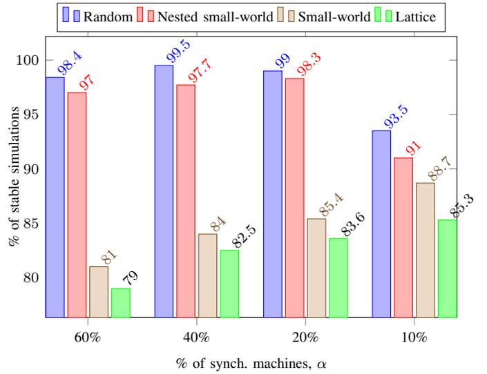
Fig. 3: Frequency stability analysis: percentages of stable, simulations following a loss of load.
