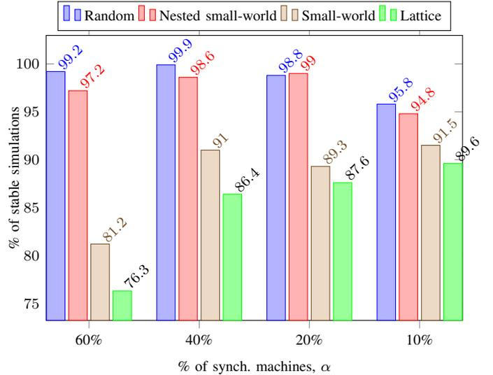
Fig. 4: Frequency stability analysis: percentages of stable, simulations following a loss of generation.
