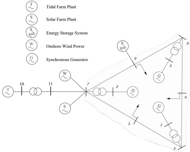
Fig. 4. The modified test power system used for the aggregated model study.
