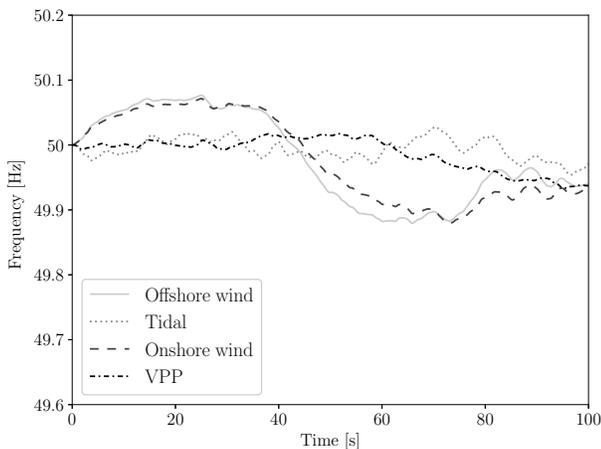
Fig. 7. The COI frequency of the system with wind/tidal turbine frequency control.
