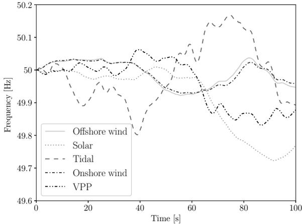
Fig. 6. The COI frequency of the system without control.
