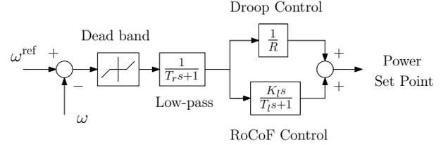
Fig. 2. The frequency control for wind and tidal turbines used in the case study.
