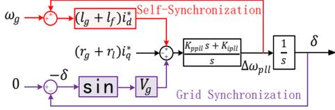
Fig. 1 Quasi-Static Large-Signal model of synchronization stability analysis.
