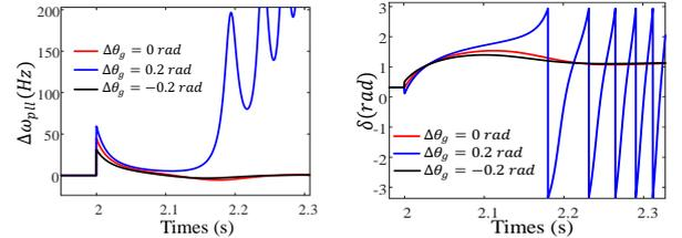
Fig. 5 Effect of the phase-angle jump.
