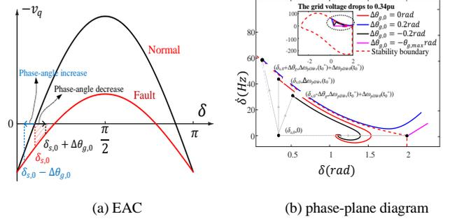
Fig. 2 Effect of the Phase-angle jump.
