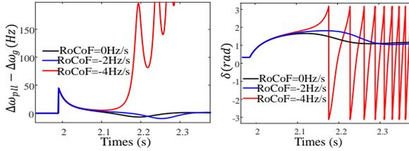
(b) The grid voltage drops to 0.337 pu and  $\Delta\omega_g = -2$  Hz.
