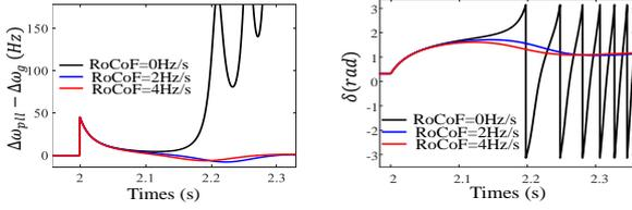
(a) The grid voltage drops to 0.334 pu and  $\Delta\omega_g = 2$  Hz.
