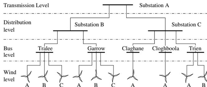
Fig. 1. Typical tree of a power grid with inclusion of wind power generation.
