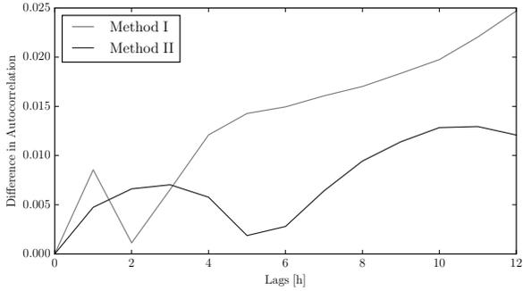
Figure 5. A comparison of the autocorrelation of Dataset 2 and the average autocorrelation of the 1,000 processes generated using Methods I and II.
