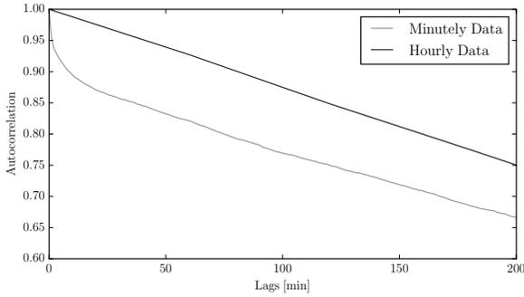
Figure 8. A comparison of the autocorrelation of the wind speed data gathered hourly and minutely in the Valentia Observatory in Kerry, Ireland [17].
