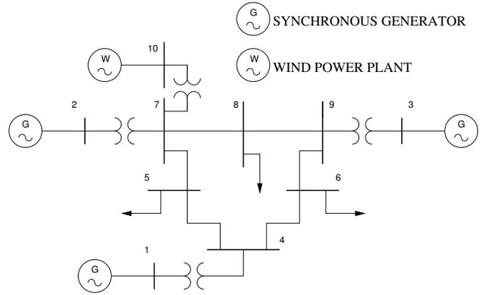
Figure 10. Modified WSCC 9-bus test system.
