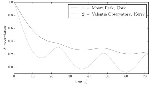
Figure 3. The autocorrelation of the wind speed datasets in Section III-A.
