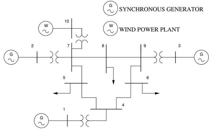
Figure 10. Modified WSCC 9-bus test system.
