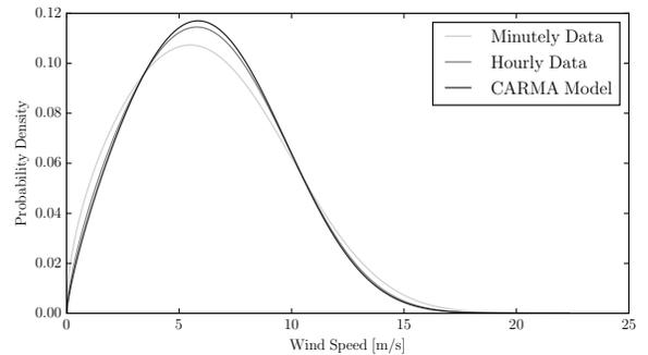
Figure 7. A comparison of the PDFs of the wind speed data gathered hourly and minutely in the Valentia Observatory, Kerry, Ireland [17]. The CARMA model PDF is the average of 1,000 simulations of the wind speed model based on the minutely data.
