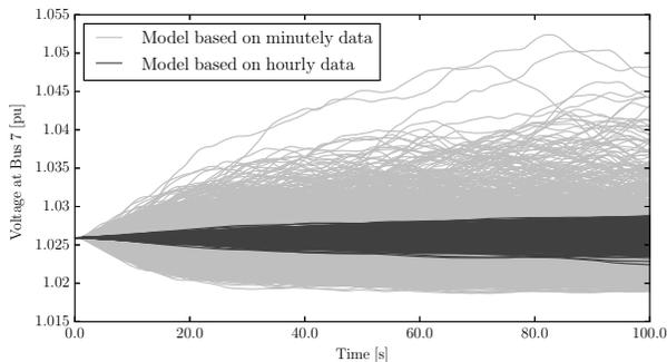
Figure 12. Voltage trajectories at Bus 7 of the test system for the 1,000 simulations using the hourly and minutely based wind speed models.
