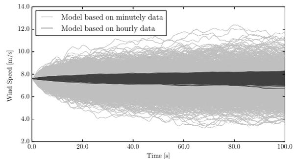
Figure 11. 1,000 generated wind speed processes based on hourly and minutely data fed to the wind power plant in the test system.
