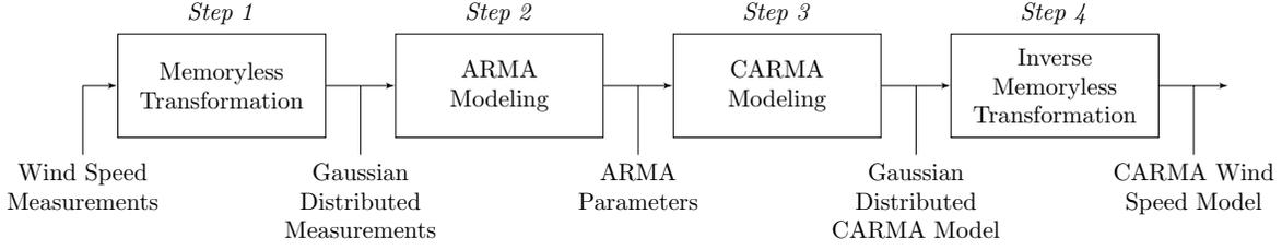
Figure 1. The four steps to construct the proposed SDE-based CARMA wind speed models.
