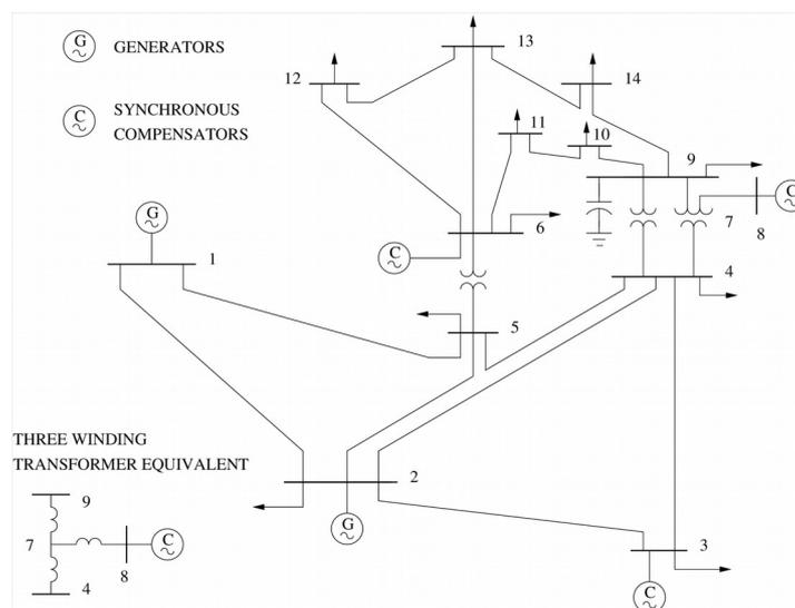
Figure 2: Single-line diagram of the IEEE 14-bus system.
