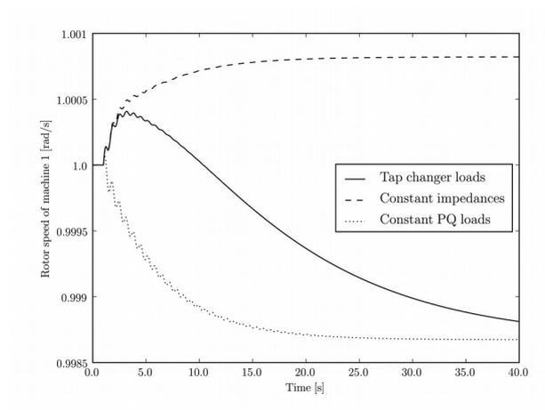
Figure 3: IEEE 14-bus system. Dynamic response following line 2-4 outage for different load models.
