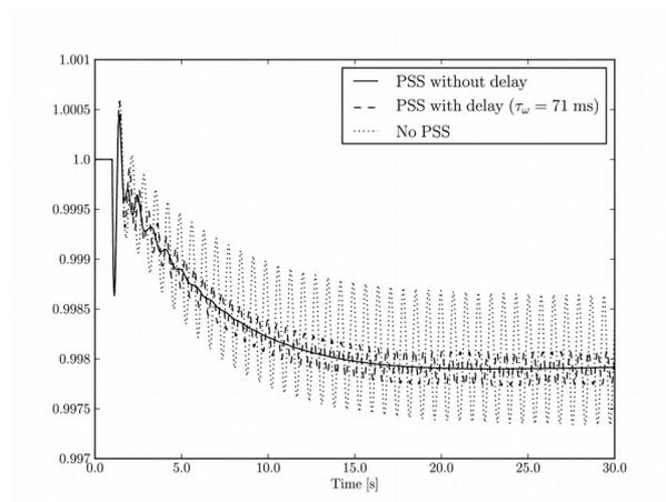
Figure 4: IEEE 14-bus system with a PSS connected to generator 1. Time domain simulation following line 2-4 outage; the case without PSS is equivalent to the case with a PSS with an infinitely delayed input signal [21].
