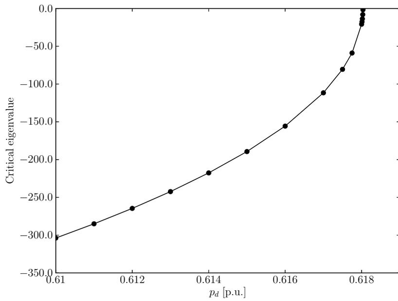
Figure 2: SMDL system without SVC: Eigenvalue loci.
