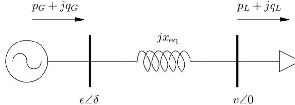
Figure 1: One-line diagram of the single machine dynamic load (SMDL) system.
