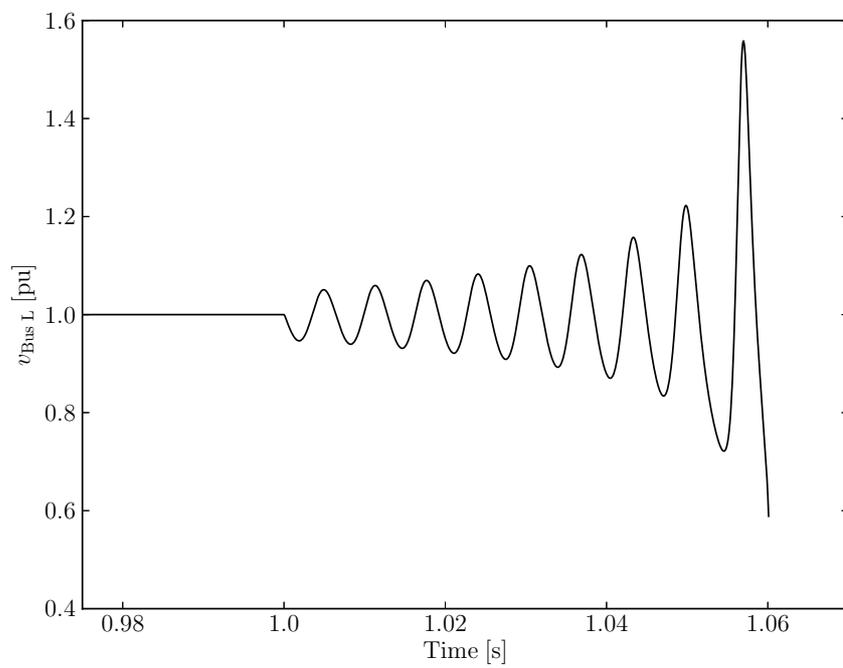
Figure 9: SMDL system with SVC: voltage collapse induced by a sudden load increase (from 1.05 to 1.09 p.u.).
