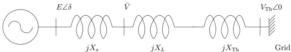
Figure 1 Synchronous machine connected to a network.
