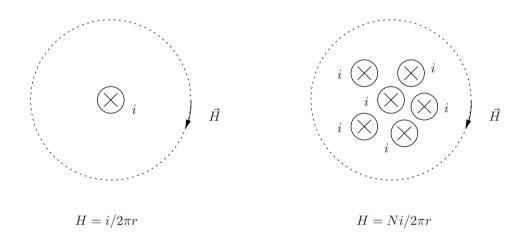
• The advange of using N turns is an easy way to *increase* the magnetic field  $\vec{H}$  while keeping relatively small the current of the winding.
