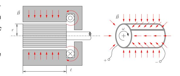
ullet The magnetic induction  $ec{B}$  is radial and time-invariant. While rotating, the coil spanned area changes its relative position with respect to the magnetic induction:
